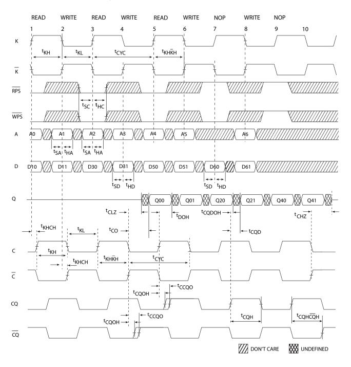
Figure 5. Read/Write/Deselect Sequence<sup>[26, 27, 28]</sup>
